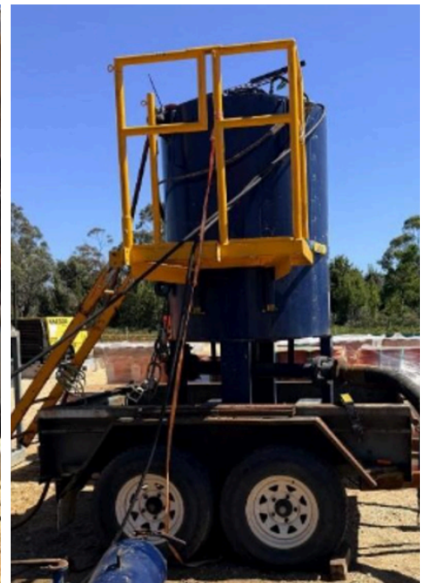
10 bbl batch tank with 0.2 bbl dead volume and agitators, hydraulically driven
