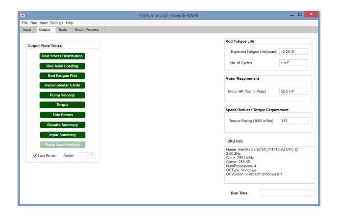
STIPumpCard contains tools, including: unit conversion, pump intake pressure estimator (from IPR curve or fluid level), stroke rate estimator from production rate, free-gas estimator (amount of free gas at intake based on gas separator used), damping factor estimator, pump efficiency and slippage calculator.
