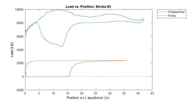
STIPumpCard outputs the fatigue loading as well as rod tensile loads.
