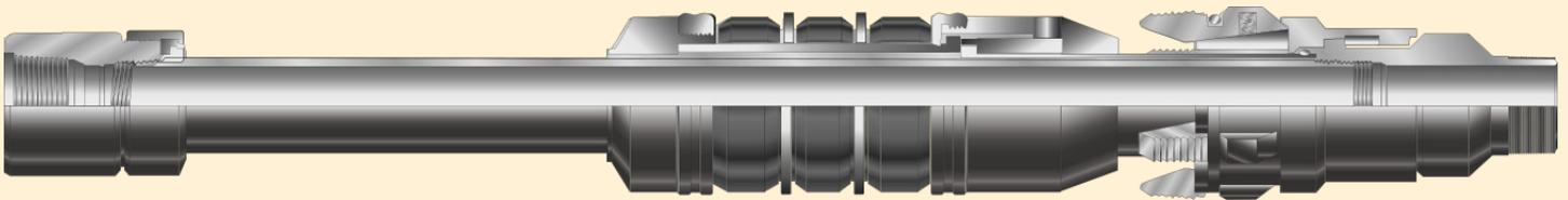
Model SR3-SG Single Grip Retrievable Casing Packers are used in production as a convention long stroke Packer. They feature a proven three element packing system and a large by-pass area through the Packer. They are available for 4" through 9-5/8" casing.
