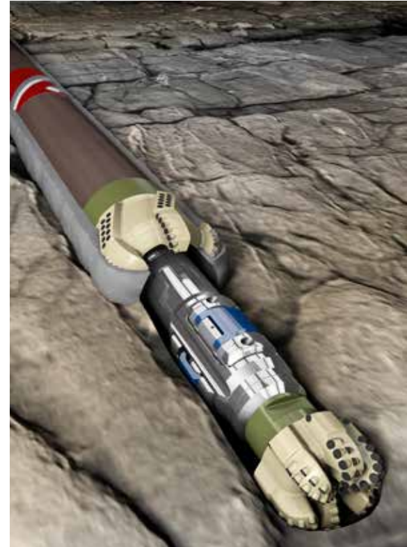
After the Direct XCD bit drills to TD, it serves as a casing shoe (left); after cementing, the bit's alloy composition allows it to be efficiently drilled out (right).
