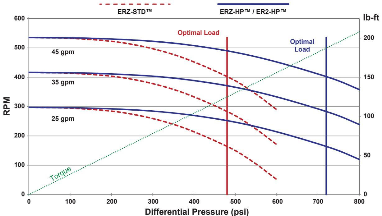
Power section performance curves are for reference only. Actual performance will vary with different downhole conditions and rotor/stator fits. If operated above the optimal differential pressure, stator life will be reduced. Optimal load power calculation is based on maximum RPM and optimal load torque. Information contained in this document is subject to change without notice. The above is referenced from a Roper Pumps® Power Section.
