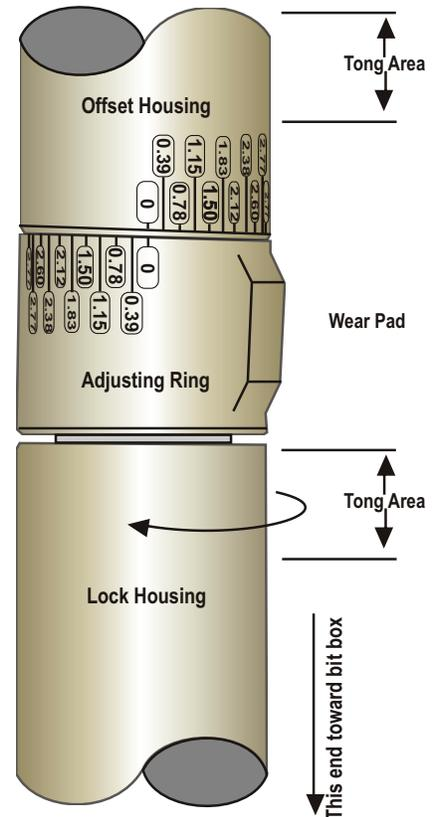
3. Slide the Adjusting Ring down to disengage the teeth in the ring and the Offset Housing.
