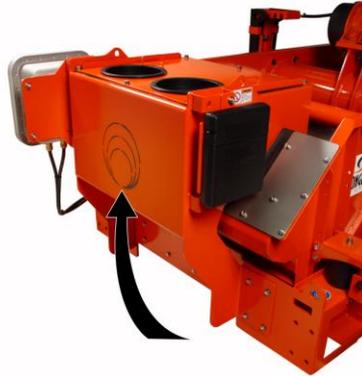
Figure 12. Piping Installation Guide Stenciling (Arrowed)
