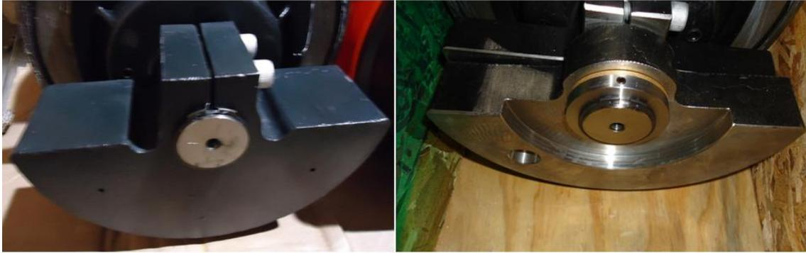
Figure 20. 50Hz Fixed Weight (Left) & Swing Weight (Right)
