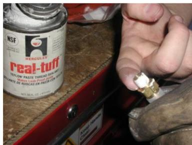
**Figure 35. Sealant Applied on a Plug Thread**
