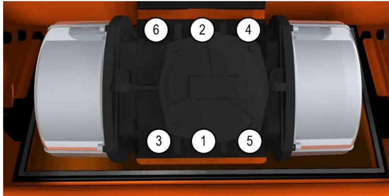
Figure 30. Motor Bolt Torque Pattern
