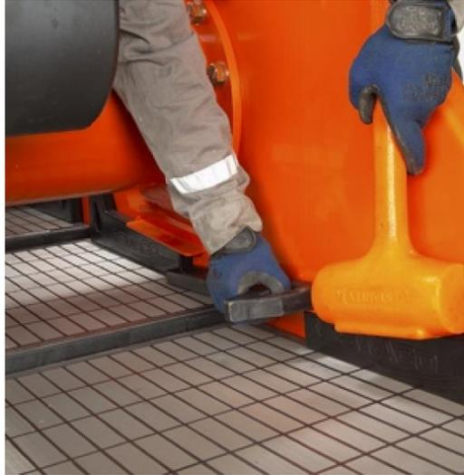
Figure 26. Use Extra Wedges with a Mallet to Loosen Screen Wedges
