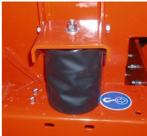
**Figure 32. Spring Enclosed in Nitrile Boot**
