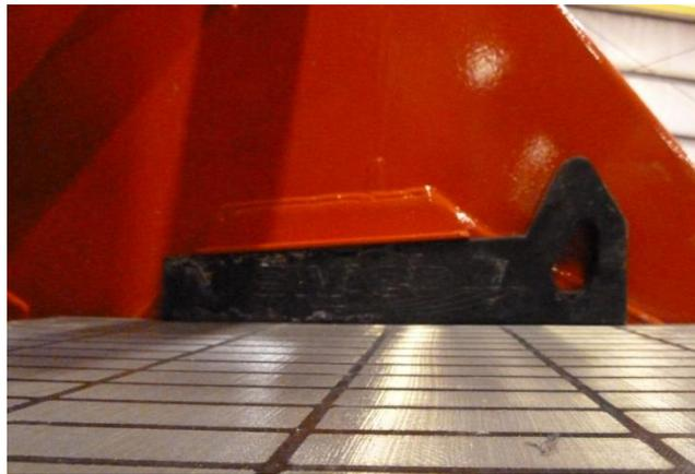
**Figure 28. Screen Wedge Secured to Unit**
