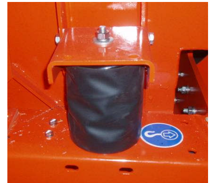
Figure 28 Spring Enclosed in Nitrile Boot
