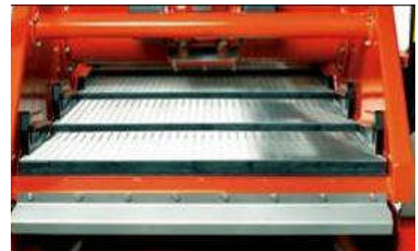
Figure 20 Screens & Wedges Firmly In Place
