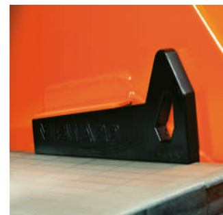
Figure 23 Wedge Positioned Between Screen Surface & Support Bar
