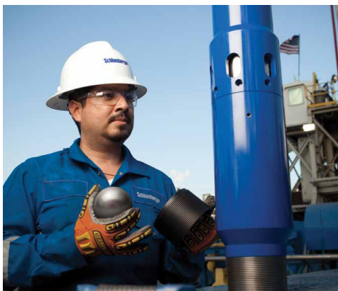
Falcon* uncemented multistage stimulation system with ELEMENTAL* degradable technology frac ball.
