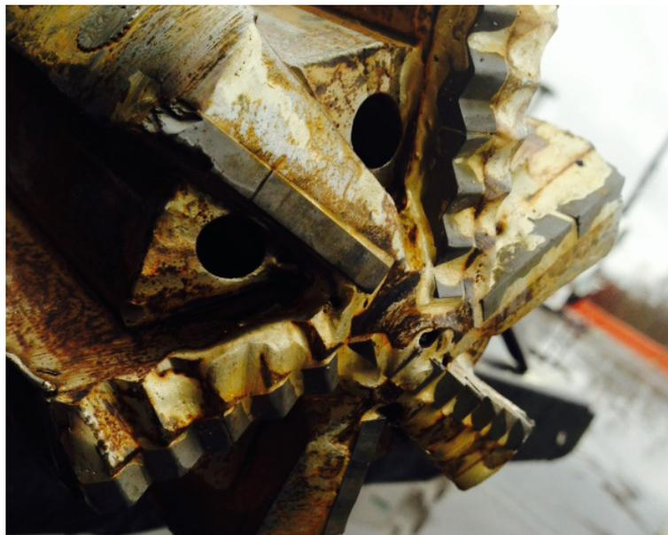
*The D2 TT Turbomill mill milled through 169 total frac plugs in one run per well at an average of 20 min per plug. This brought the time to mill Copperhead frac plugs from 3.5 h to 30 min. The new mill also decreased the time to mill Diamondback frac plugs by 17%. These efficiencies saved the operator an average of 5 hours and USD 8,000 per well.*
