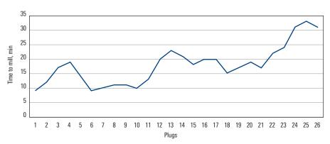
On average, the plugs were milled 12 minutes faster per plug compared with the planned time.
