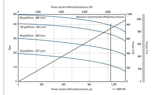
Operating a power section above the maximum recommended differential pressure will reduce stator life. Performance Curves are recorded at 73 degF on a STD fit Rotor/Stator combination and are for reference only. Actual power section performance may vary depending on the down hole temperature and rotor/stator fit. Performance data are subject to change without notice. Power calculation is based on maximum RPM at full torque. Stator sizes subject to change without notice.
