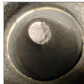
WT —Minor wear (Level 2 severity).
