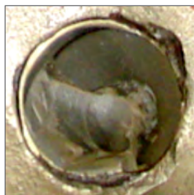
DL —Stinger element delamination.
