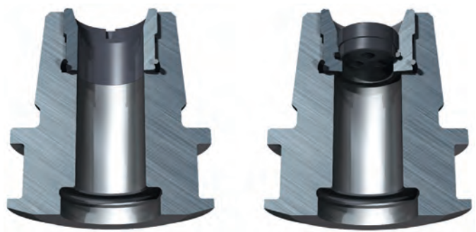
6 5 / 8 -in API pin restrictor assembly with nozzles.
