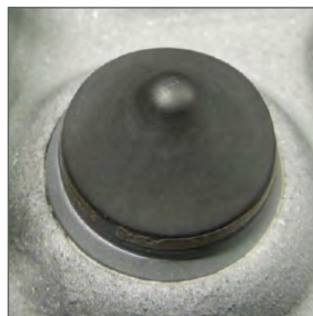
WT —No wear (Level 0 severity).
