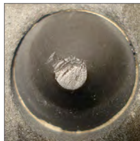
WT —Minimal wear (Level 1 severity).
