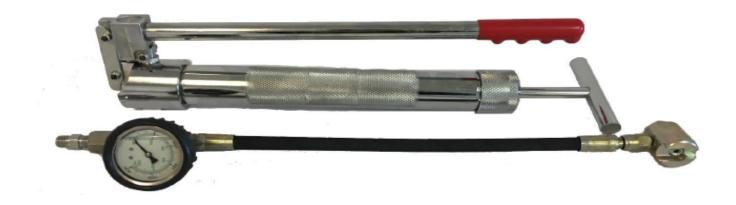
Part# SPG-02 - Includes a built-in safety check valve, ½" high pressure tee, 15,000 psi gauge with cover, 18" high pressure hose, and a giant button head coupler with steel button.
