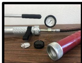
**Step 7:** Remove the cartridge loader and install the hose assembly on the grease barrel, tight.
