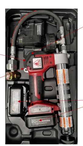
C) 1 and 2 Switch allows two flow rates. You can switch it to 1 to 4 ounces per minute or 2 to 6 ounces per minute.
